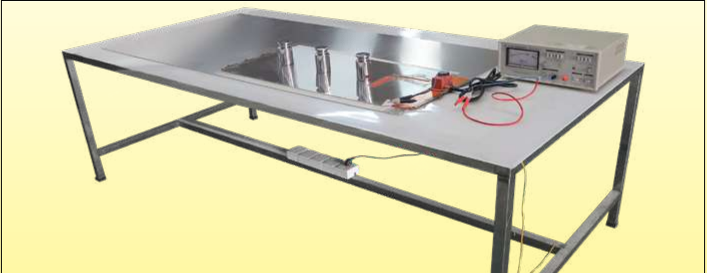
Device for measuring the insulation resistance. The measured values are always greater than 0.1Gohm
