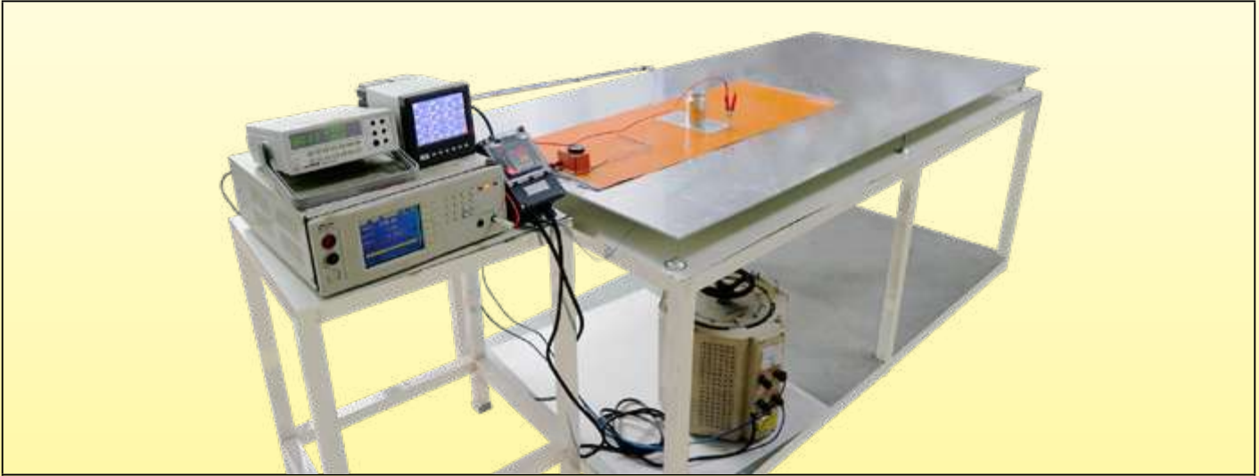
Measuring equipment for total current leakage at hot condition
